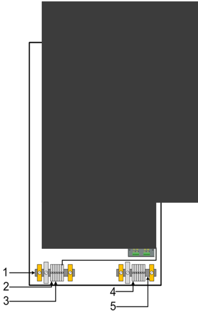
Figure 6 Typical safety ground connections in Series 8 cabinet
